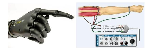
Producing such a robotic arm can use signal from the brain (e.g., electroencephalography (**EEG**)) or signal from the healthy part of the hand **EMG** (electromyography). EMG is a technique for evaluating and recording the electrical activity produced by skeletal muscles. Using non-invasive EMG a robotic hand can be controlled (Maier, Sebastian and Smagt van der, Patrick 2008).
