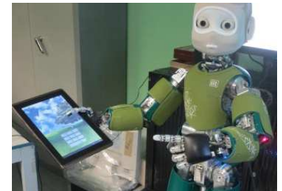
Figure 1: Example of a pointing gesture performed by the iCub robot Nina at GIPSA-Lab.
